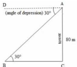
$$\begin{aligned}\tan 30^\circ &= \frac{AC}{BC} \\ \Rightarrow \tan 30^\circ &= \frac{80}{BC} \\ \Rightarrow BC &= \frac{80}{\tan 30^\circ} = \frac{80}{\left(\frac{1}{\sqrt{3}}\right)} \\ &= 80 \times 1.73 = 138.4 \text{ m}\end{aligned}$$
