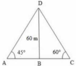
$$\begin{aligned}\tan 45^\circ &= \frac{BD}{BA} \\ \Rightarrow 1 &= \frac{60}{BA} \\ \Rightarrow BA &= 60 \text{ m} \quad \dots (1)\end{aligned}$$
